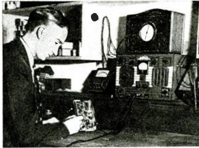
The author is here shown using the Rimco Dynalyzer (this is the instrument in the photo to which the test cord is connected).
