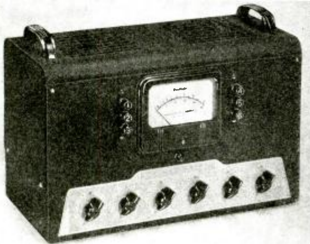
Fig. 1. The front-view photo of the completed hi-fi recording-playback sound amplifier, showing the cover in place; the various controls are identified as follows: pushbuttons (at left of the decibel meter, top to bottom)—Playback, Dialogue Filter, Record; (right) 0 Db., +20 Db., +30 Db. Bottom row of controls (left to right)—Mikes Nos. 1 & 2, Playback, Master Gain, H.F. & L.F. Controls.
